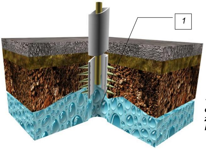
1-lifting of the cone of water in zone of perforation interval
